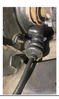
For aluminum bell slide the cover in place as shown below.
