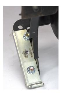
Pass the lower end of the clutch cable through the clutch rod hole in the firewall near the steering column. A hole may need to be cut in the rubber for automatic cars.
