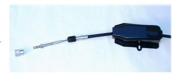
Fasten the cable to the floor with the P-clamp provided so the cable will not come in contact with the exhaust system. Rely on the p-clamp being installed to help align the cable coming straight into the clutch fork. The P-clamp will be loose enough to allow the cable housing to move.
